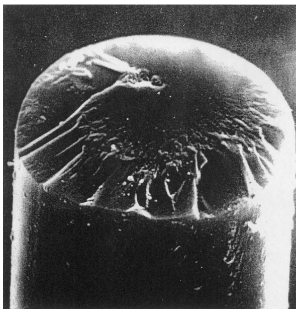
Fig. 1. Fracture morphology of a first generation Nicalon fibre, having a diameter of 15 \mu\text{m} and revealing a glassy appearance.
