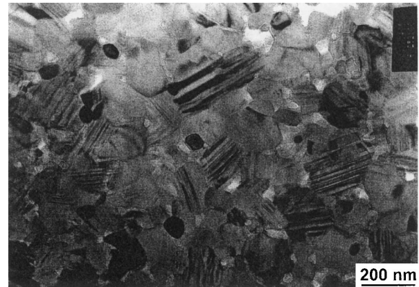
Fig. 8. The microstructure of the Sylramic, near stoichiometric SiC fibre, revealing SiC grains of around 200 nm, \text{TiB}_2 grains of 50 nm and free turbostratic carbon at triple points.
